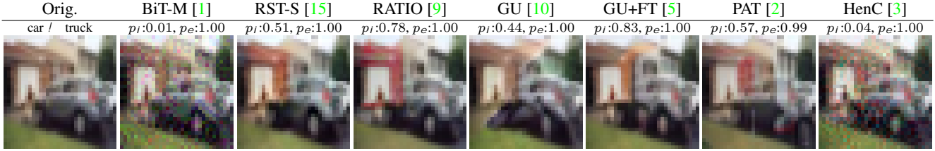
Figure 2. CIFAR-10 : l_2 -VCEs of radius \epsilon = 2.5 of different classifiers for the change “car \rightarrow truck”. We denote by p_i resp. p_e the confidence in the target class for the original image and the generated VCE. All generated VCEs are valid as high confidence in the target class is achieved but only adversarially robust models, see Tab. 1, show class-specific changes.
